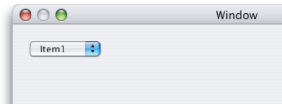
Figure 7-32 The popup button after checking the Small checkbox
