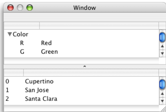
Figure 3-6 A split view that contains an outline view and a table view
