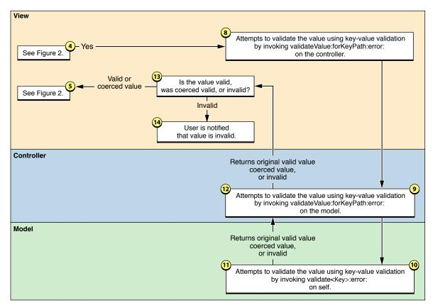
As in ""Changing the Value of a Model Property" (page 47)" this specific example is of an NSTextField with its value binding bound to an NSObjectController's selection using the selection.firstName key path. The NSObjectController's content binding is bound to a model object that encapsulates a person's name and address.
