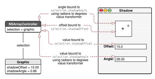
The text fields' values are bound to the angle and offset of the graphic object's shadow; the joystick provides a graphical representation of angle and offset. The angle in the text field is displayed in degrees, and the angle used internally by the joystick is specified in radians. The bindings for both of these specify a reversible value transformer that converts between radians and degrees.
