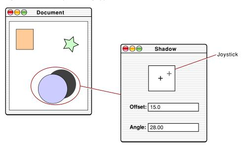
The implementation of the inspector is illustrated in Figure 2. Both the text fields and the joystick are bound to the selection of an NSArrayController. The controller's contentArray is bound to an array of Graphic objects. A Graphic has instance variables to represent its shadow's angle in radians and its offset from its center.
