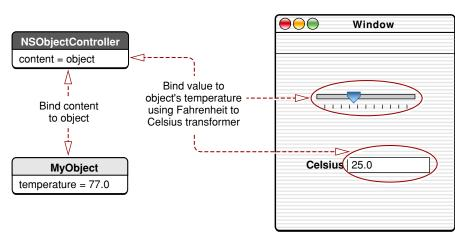
Figure 5 Displaying temperature using transformers
