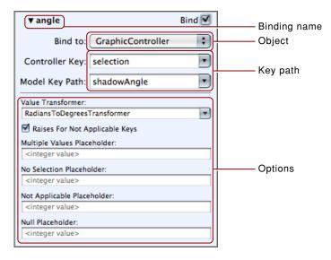
Establishing this binding in Interface Builder is equivalent to programatically sending this message to the joystick:
