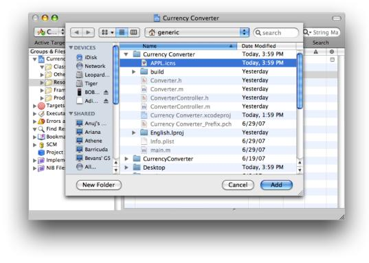
Figure 7-7 Selecting the icon file to add to the Currency Converter project
