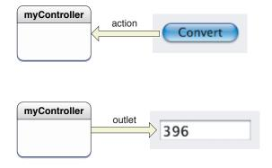
In the Actions column (in the Connections pane of the inspector), all action methods are defined by the class of the target object and known by Interface Builder. Interface Builder identifies action methods because their names follow this syntax:
