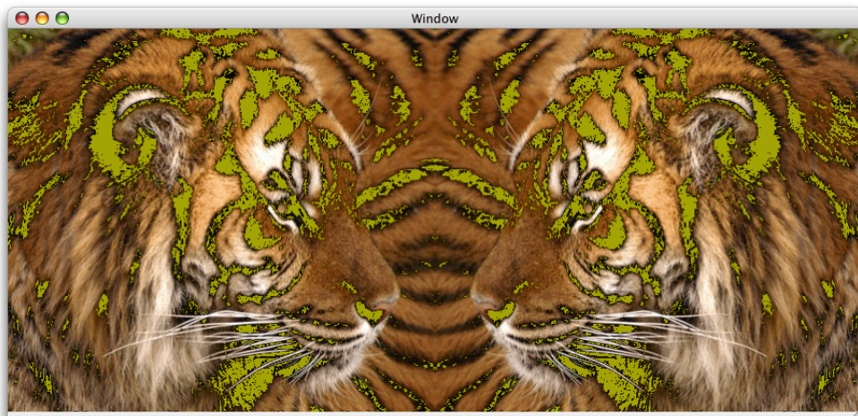
Figure 11-13 An image drawn after masking a range of colors and setting a fill color
