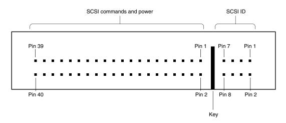
Table 2-2 lists the interface signals for the 40-pin segment of the connector.
