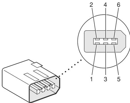
**Table 3-2** Pin assignments on the FireWire 400 connector
