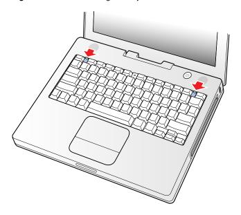
**Important:** When reinserting the keyboard, make sure the latches at the top line up with the corresponding slots in the case and that the bottom tabs are aligned correctly and completely seated before tilting the keyboard into place. See Figure 3-6 (page 40).
