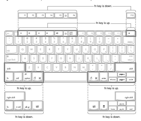
Figure 3-9 Embedded numeric keypad operation
