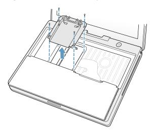
Once the RAM expansion module has been installed in the slot, close up the computer by performing these steps in reverse order.
