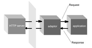
Figure 14. Request-Response Loop: Application and Server Level
