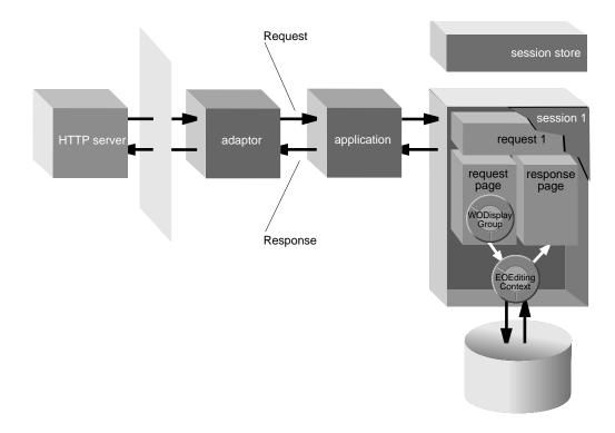
Figure 18. Request-Response Loop: Database Access
