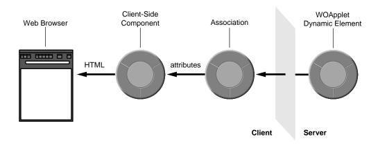
Figure 13. Client-Side Java Components
