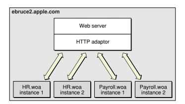
Figure 4-1 Deployment on one computer, using one adaptor
