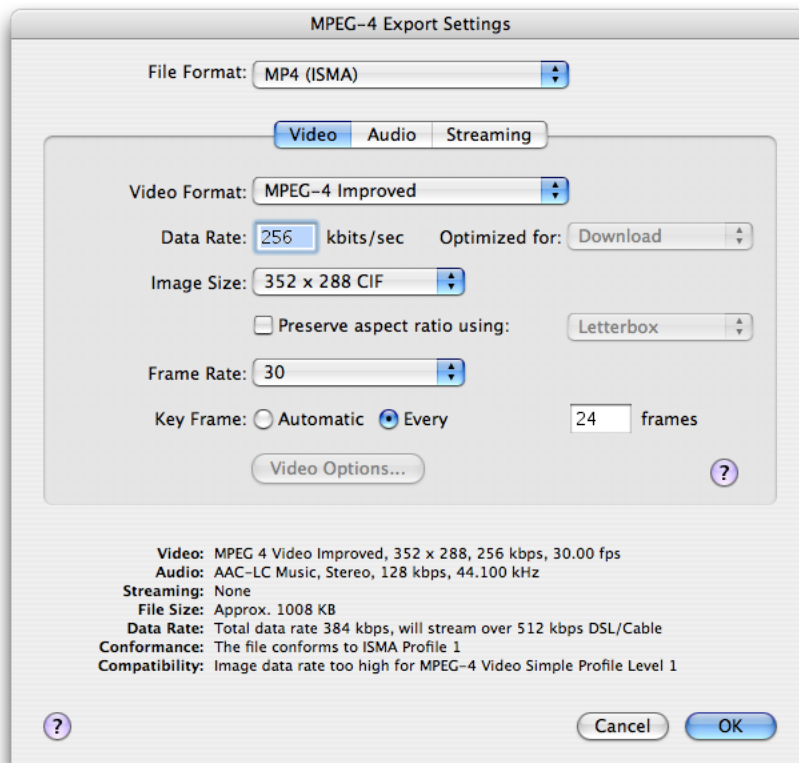
Figure 1-9 MPEG-4 export settings dialog with a Preserve aspect ratio checkbox
