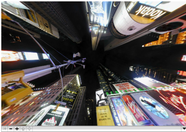
Figure 2-1 A cubic panorama movie in QuickTime with standard controls that let users tilt up and down 180.0 degrees
