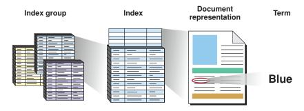
At the outermost level, as shown in the figure on the left, an application typically works with a group of indexes. An individual index, depicted in the figure under the heading "Index" and represented in Search Kit as an SKIndexRef opaque type, contains representations of one or more documents.
