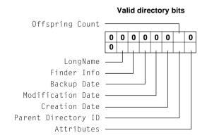
Figure 1-12 shows the valid file bits. The FPCatSearch command can search for this information only when it searches for files.
