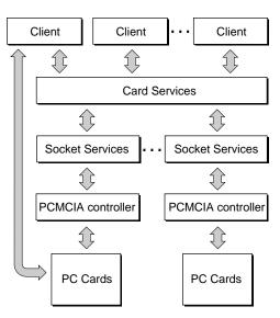
Note: Each client may communicate directly with the PC Card(s) installed
